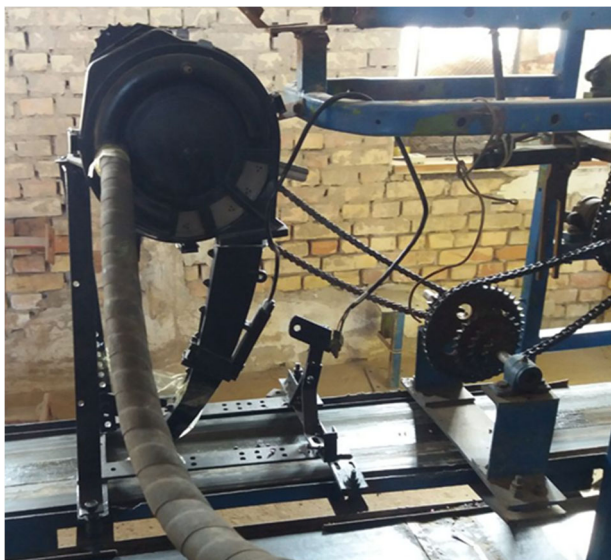
Fig. 1. Case-an overview of a laboratory stand equipped with a pneumatic seed drill 1200.
