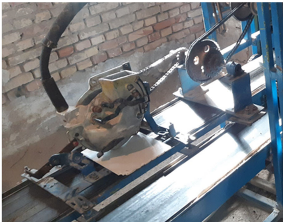
Fig. 3. Laboratory stand with pneumatic planting machine PS-4 seeder.
